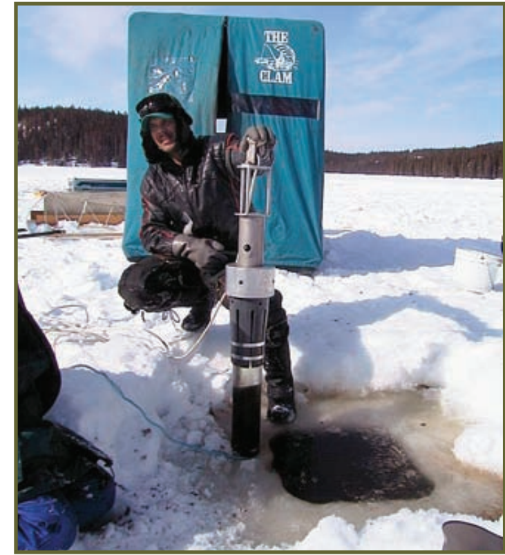
A technician prepares to take a lake bottom sediment core through the lake ice in winter.
